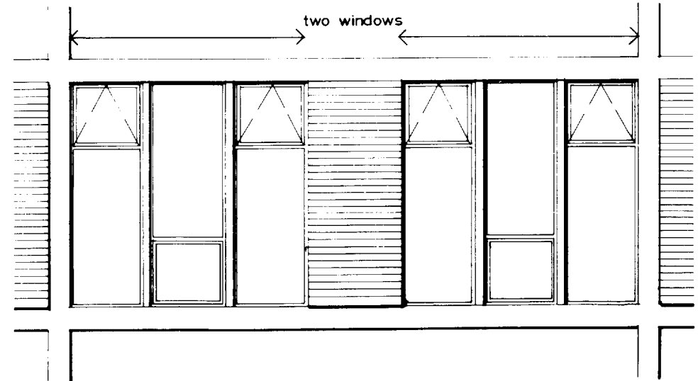
3.4 The assembly is most sensibly regarded as having two window components, each being the largest single composite item within the supply of one manufacturer
